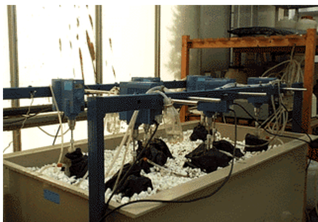
Figure 1. 20L reactors using in the co-digestion experimental trials.
